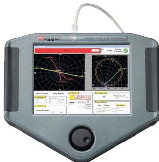
Current transformers can be tested in their equipment configuration, such as being mounted in transformers, oil circuit breakers or switchgear. It is necessary for the equipment to be completely isolated from the electrical system prior to testing.
